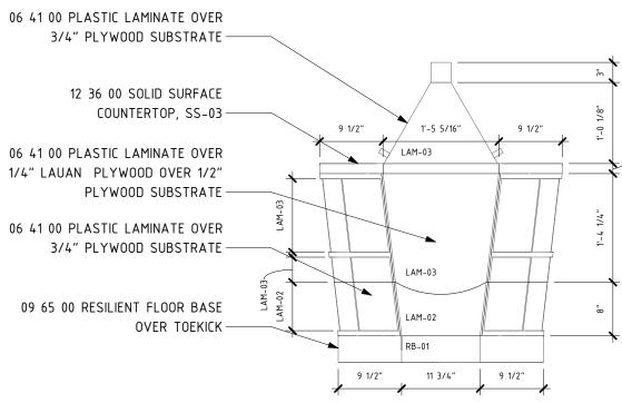
12 36 00 SOLID SURFACE COUNTERTOP, SS-03-06 41 00 PLASTIC LAMINATE OVER 1/4" LAUAN PLYWOOD OVER 1/2" PLYWOOD SUBSTRATE -
