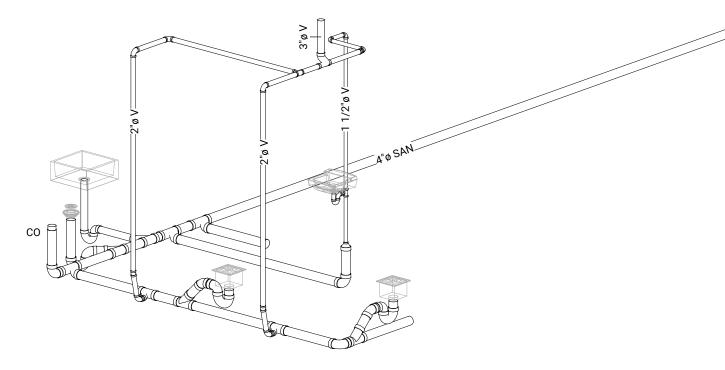
PLUMBING RISER DIAGRAM - SANITARY & VENT PIPING NO SCALE
