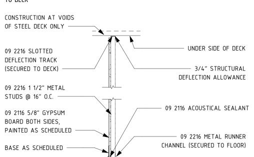
W5: LIGHT GAUGE FRAMING INFILL WITH PAINTED GYPSUM WALLBOARD BOTH SIDES
