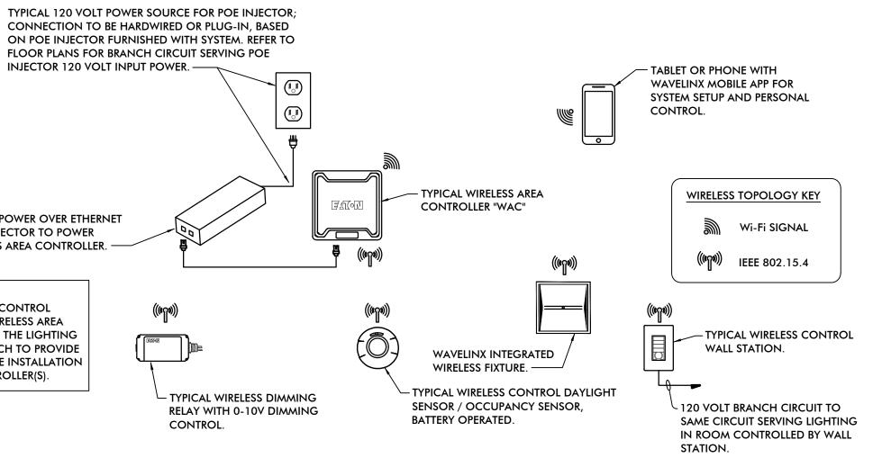
WIRING DIAGRAM SHOWN IS BASED ON A WIRELESS LIGHTING CONTROL SYSTEM MANUFACTURED BY COOPER; THE COOPER "WAVELINX PRO" SYSTEM. SYSTEMS FROM "EQUAL"
